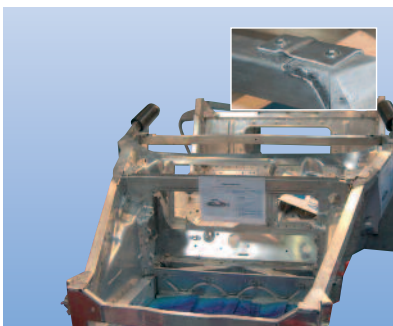
A (5:1) Visual check that stem has been locked during setting (see specific nosepiece on page 39/41)
