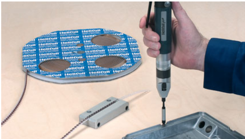
Installation of HELICOIL® Plus
